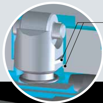
Sealing land of piston not yet get connected with counter seal point of anvil, i.e. oil flows freely in between.
